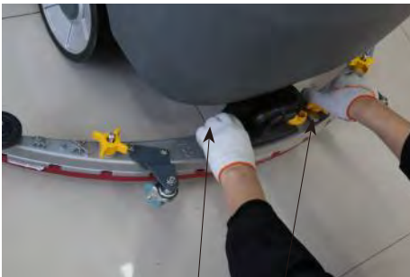
Unscrew the fixing nut counterclockwise
